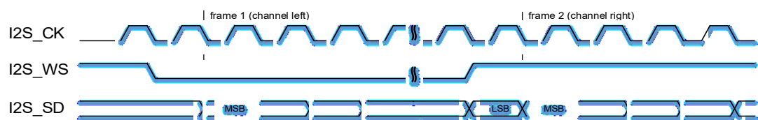
Figure 21-14. I2S Philips standard timing diagram (DTLEN=00, CHLEN=0, CKPL=0)
