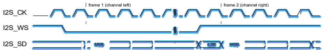
Figure 21-16. I2S Philips standard timing diagram (DTLEN=10, CHLEN=1, CKPL=0)
