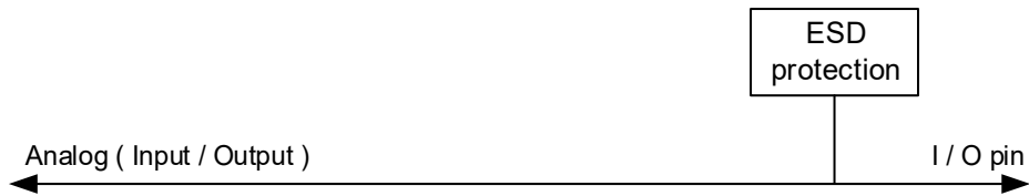
Figure 7-4. Basic structure of Analog configuration
